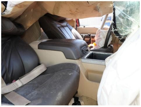
The photographs of those "Super Duty" trucks shown above do not show the full extent of the intrusion of the roof into the occupant compartment; the intrusion was greater than the photographs indicate. It is the nature of metal that the dynamic crush exceeds the static crush—the metal roof rebounds from the full extent of the crush that occurs in the rollover wreck.
