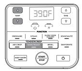
2 Use the up and down TIME arrows to set the cook time in minute increments up to 1 hour. 5-minute increments from 1 hour to 4 hours.
