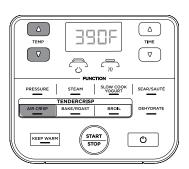
2 Use the up and down TIME arrows to set the cook time in minute increments up to 1 hour.
