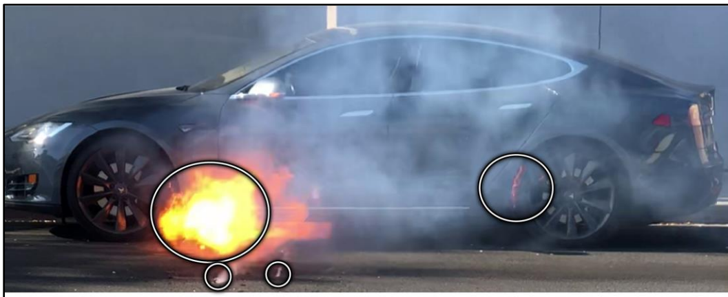
Figure 13. Image from bystander's video with fire visible behind left front wheel and in left rear wheel well. (Source: Los Angeles County Sheriff's Department)
