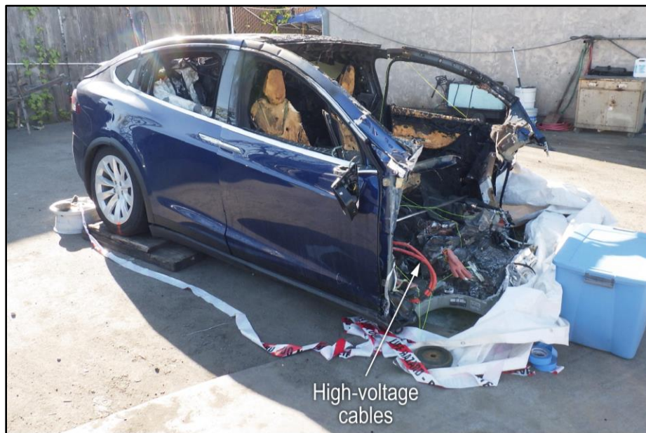
Figure 8. Damaged SUV with exposed orange high-voltage cables forward of front seat.
