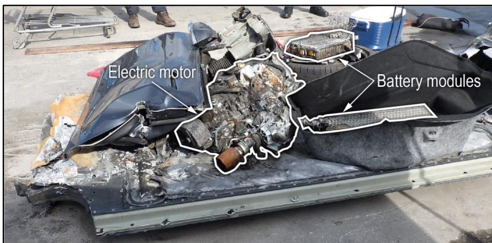
Figure 11. Debris pile on pallet with remains of electric motor and battery modules highlighted.
