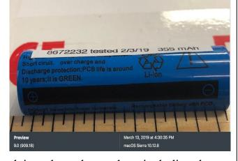
90. Amazon makes numerous false claims about the product, including that the battery has a capacity of 5000 mAh, when it tested at only 355 mAh. The batteries
