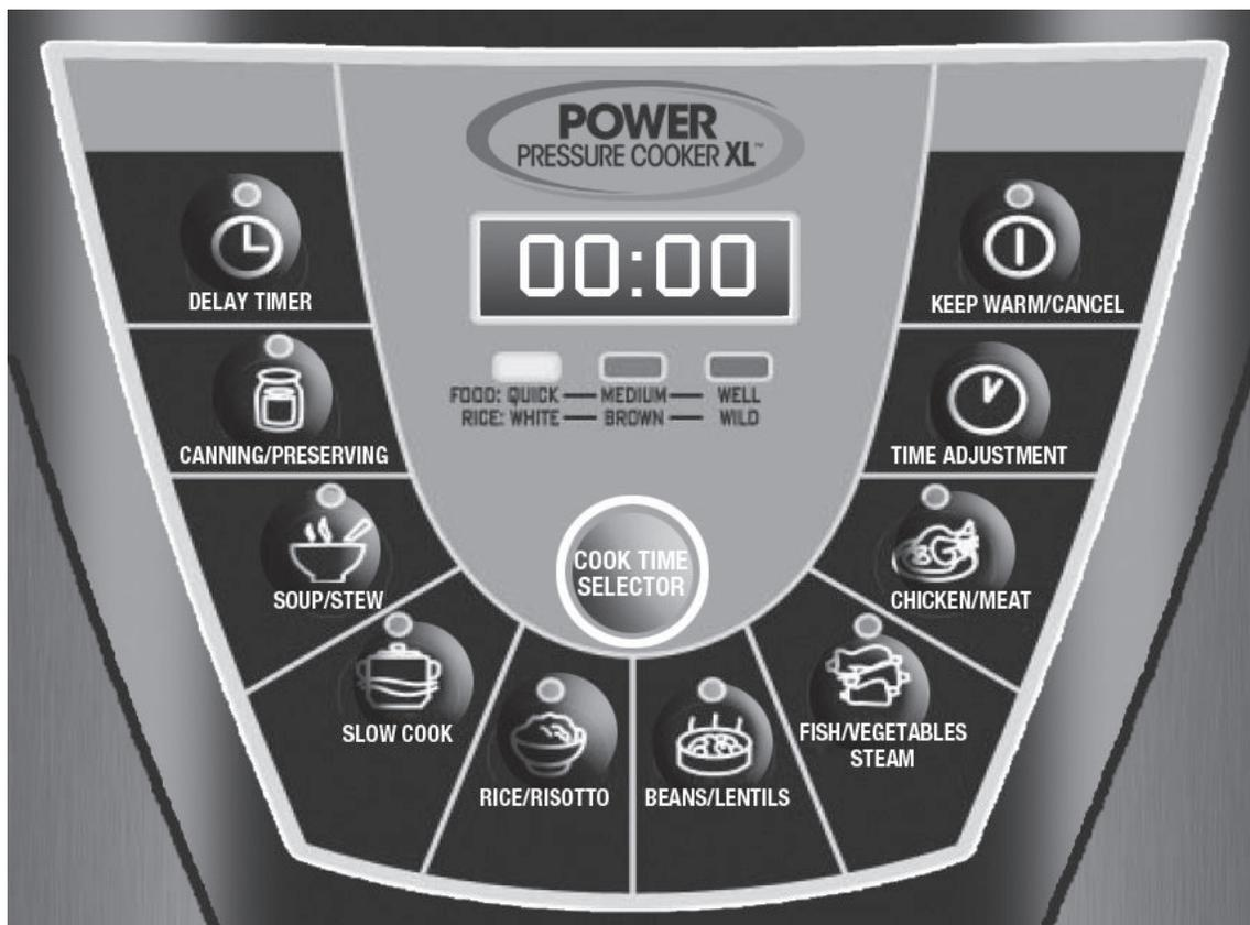
The Power Pressure Cooker XL has seven basic cooking modes that may be used alone or in combination to produce an infinite variety of results.
