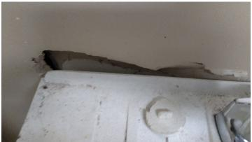
e. ... The entire top of the unit separated and flew across the room exploding that [sic] glass across the laundry room and into our hallway, and the explosion put holes in the wall, damaged shelves, etc. If my wife or son were in the room when this happened, I have no doubt that they would be in the hospital or possibly even killed. (Report date: November 18, 2015; Model No.: WA50F9A6DSW/A2; Photographs Below)
