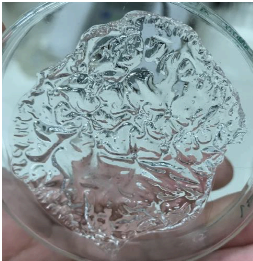
13 14 15 Figure 2: Striations on gel caused by rapid cooling and oxygenation of pre gel solution.
