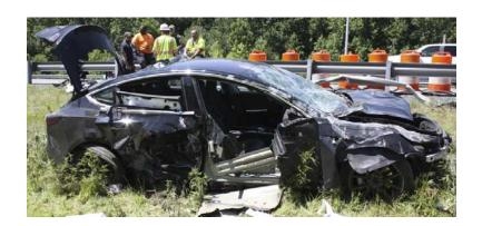
18. In the accident, none of the subject Model 3 airbag's deployed, not even its passenger side airbag.
